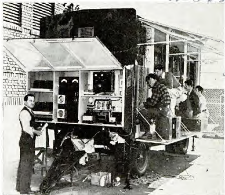
If enemy bombs disrupt lines, this switchboard can serve 400 telephones
